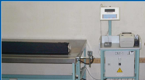
laser measuring and check weighing of textile rolls
