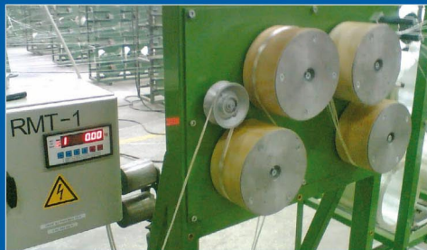
examples of ALYA test kits for bending strength and tensile forces
