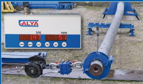
examples of ALYA test kits for bending strength and tensile forces
